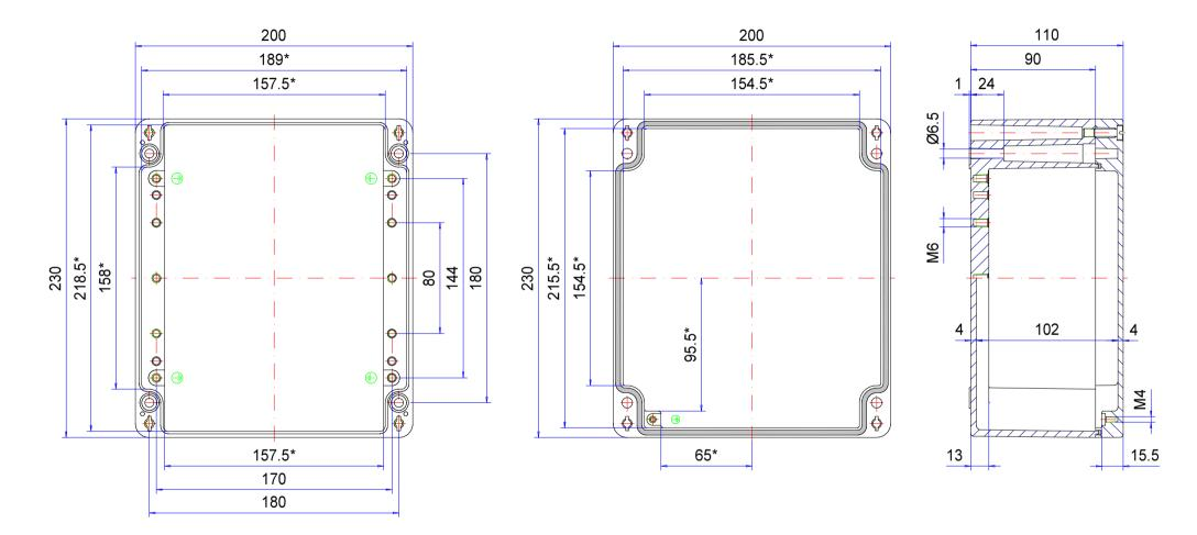
\* Please note: Mould slope for casting ejection, dimensions in the amount of the bottom!
