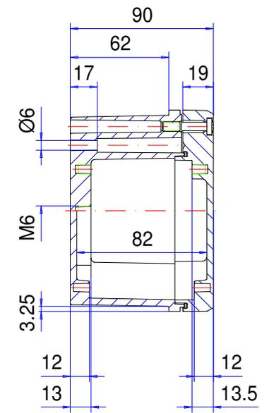
\* Please note: Mould slope for casting ejection, dimensions in the amount of the bottom!
