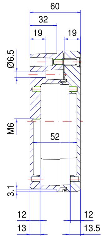
\* Please note: Mould slope for casting ejection, dimensions in the amount of the bottom!
