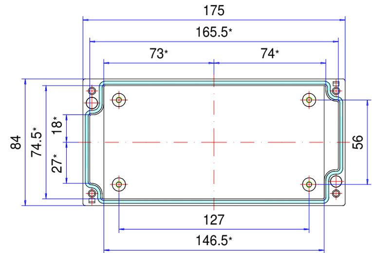
\* Please note: Mould slope for casting ejection, dimensions in the amount of the bottom!
