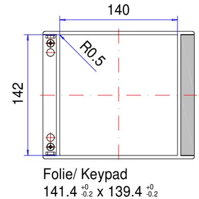
\* Please note: Mould slope for casting ejection, dimensions in the amount of the bottom!
