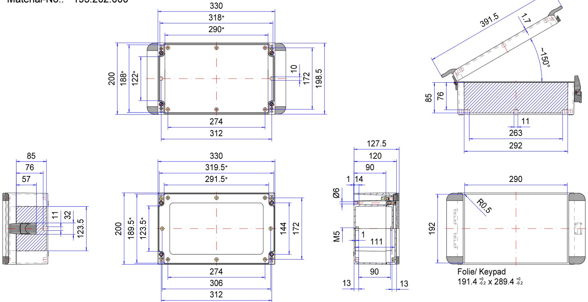
\* Please note: Mould slope for casting ejection, dimensions in the amount of the bottom!
