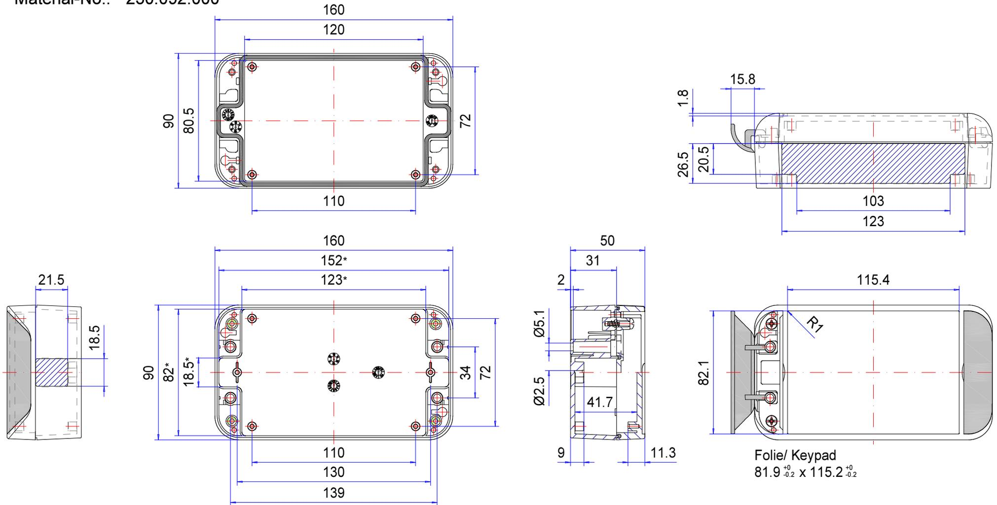
\* Please note: Mould slope for casting ejection, dimensions in the amount of the bottom!
